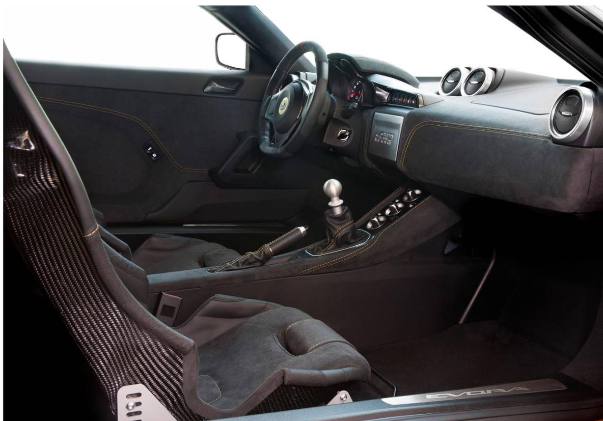
The rest of the Sport 410's cabin has received attention as part of its development. Weight saving measures includes attractive one-piece door trim panels finished in Alcantara®, with contrast stitching, the deletion of door arm rests and stowage pockets, the relocation of tailgate and fuel filler release buttons and the removal of speakers - if an entertainment system is not specified.
