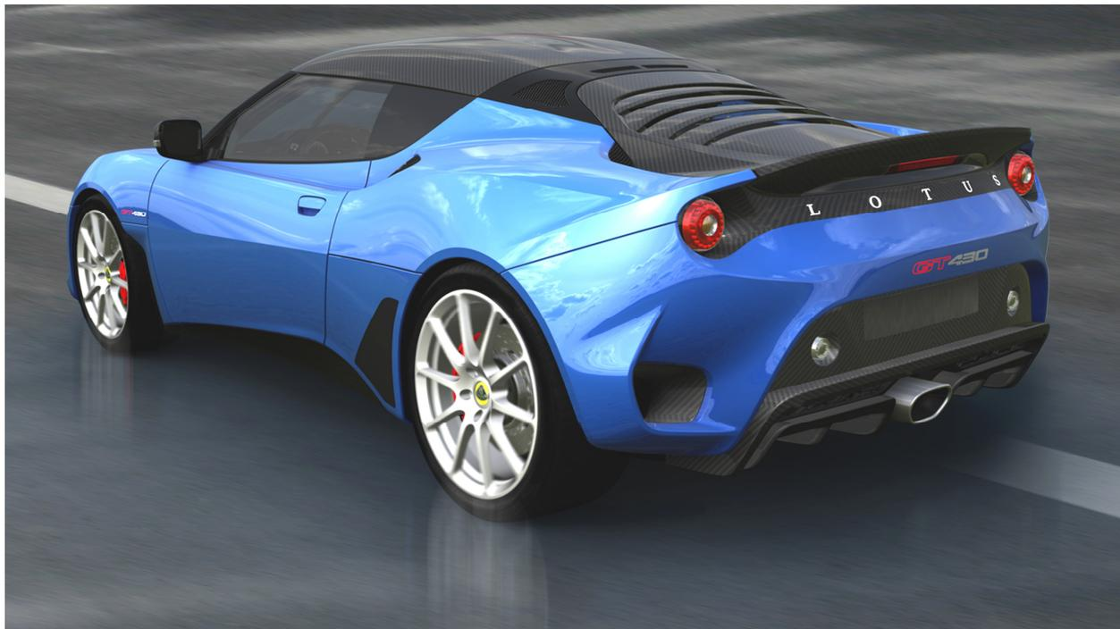
The Evora GT430 is differentiated from the Evora GT430 Sport through the inclusion of motorsport derived aerodynamics provided by a carbon fibre splitter, a large, profiled carbon wing and louvers on top of each front wheel arch which reduce pressure within the front wheel arches together with wider wheels and tyres.
