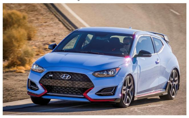
In profile, exclusive N-design rocker side sills and available lightweight 19-inch alloy wheels with a machined-finish dual-spoke star design clearly differentiate the N model from other Veloster models. Tires are of the ultra-high performance category, with standard 225/40R18 Michelin Pilot SuperSport summer tires for the 18-inch wheel design and exclusive-compound 235/35R19 Pirelli P-Zero summer tires for the available 19-inch alloy wheel.
